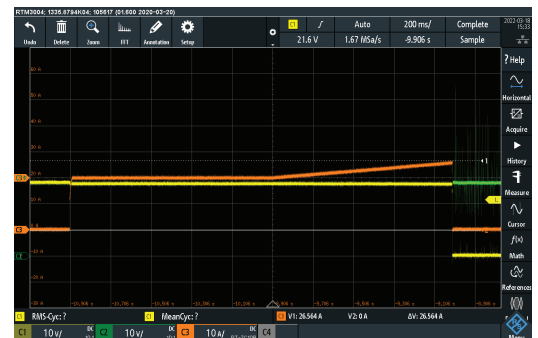
Figure 2: Output voltage waveform (yellow), with increasing output current (orange) starting from 20 A up to 28 A when INH is connected to DIS externally so that overcurrent and short circuit protections are enabled
