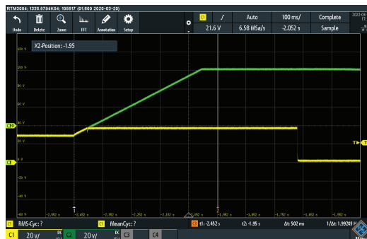
Figure 1: Output voltage clamping waveform (yellow), with increasing input voltage (green) starting from 28 VDC up to 100 VDC
